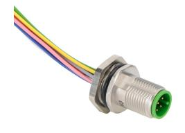
Murrelektronik bulkhead connector, M12 8-pin male to pigtail, 24 AWG, 3.2ft/1m cable length, nylon 12 conductor insulation material, IP67.
