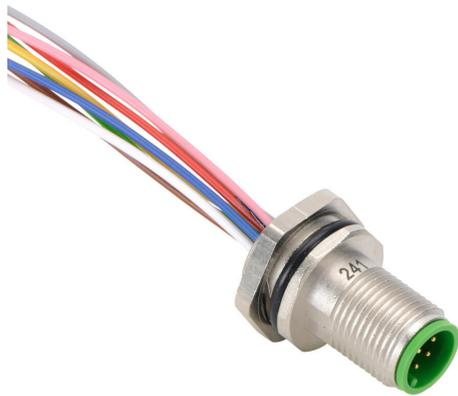
Murrelektronik bulkhead connector, M12 8-pin male to pigtail, 24 AWG, 1.6ft/0.5m cable length, nylon 12 conductor insulation material, IP67.
