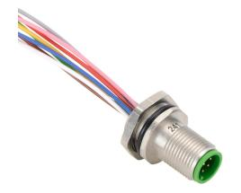
Murrelektronik bulkhead connector, M12 barrel 8-pin male to pigtail, 24 AWG, 1.6ft/0.5m cable length, polypropylene conductor insulation material. Mounting nut(s) included.
