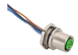
Murrelektronik bulkhead connector, M12 nut 5-pin female to pigtail, 22 AWG, 3.2ft/1m cable length, polypropylene conductor insulation material. Mounting nut(s) included.
