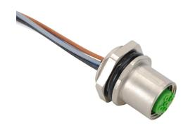
Murrelektronik bulkhead connector, M12 5-pin female to pigtail, 22 AWG, 1.6ft/0.5m cable length, nylon 12 conductor insulation material, IP67.
