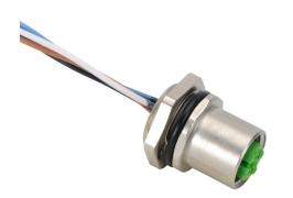
Murrelektronik bulkhead connector, M12 4-pin female to pigtail, 22 AWG, 3.2ft/1m cable length, nylon 12 conductor insulation material, IP67.
