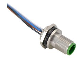
Murrelektronik bulkhead connector, M12 5-pin male to pigtail, 22 AWG, 3.2ft/1m cable length, nylon 12 conductor insulation material, IP67.
