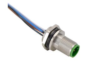
Murrelektronik bulkhead connector, M12 barrel 5-pin male to pigtail, 22 AWG, 3.2ft/1m cable length, polypropylene conductor insulation material. Mounting nut(s) included.
