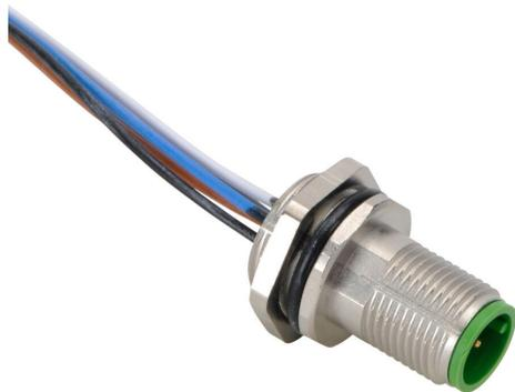
Murrelektronik bulkhead connector, M12 5-pin male to pigtail, 22 AWG, 3.2ft/1m cable length, nylon 12 conductor insulation material, IP67.
