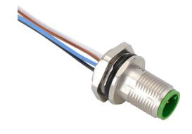
Murrelektronik bulkhead connector, M12 barrel 4-pin male to pigtail, 22 AWG, 3.2ft/1m cable length, polypropylene conductor insulation material. Mounting nut(s) included.
