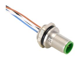
Murrelektronik bulkhead connector, M12 4-pin male to pigtail, 22 AWG, 1.6ft/0.5m cable length, nylon 12 conductor insulation material, IP67.
