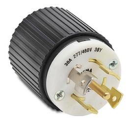
Bryant industrial heavy duty locking blade plug, 30A, 277/480 VAC, 3-phase, 4-pole, 5-wire, NEMA L22-30, accepts cord size 0.46-1.15in, nylon housing, black and white.
