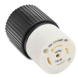
Bryant industrial heavy duty locking blade connector, 30A, 277/480 VAC, 3-phase, 4-pole, 5-wire, NEMA L22-30, accepts cord size 0.46-1.15in, nylon housing, black and white.
