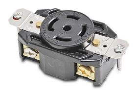
Bryant industrial heavy duty single locking blade receptacle, 30A, 277/480 VAC, 3-phase, 4-pole, 5-wire, NEMA L22-30, nylon molded housing, black.
