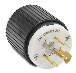
Bryant industrial heavy duty locking blade plug, 20A, 277/480 VAC, 3-phase, 4-pole, 5-wire, NEMA L22-20, accepts cord size 0.46-1.15in, nylon housing, black and white.
