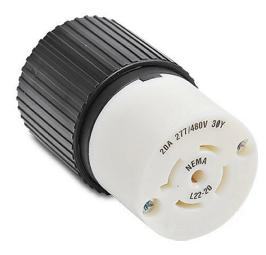
Bryant industrial heavy duty locking blade connector, 20A, 277/480 VAC, 3-phase, 4-pole, 5-wire, NEMA L22-20, accepts cord size 0.46-1.15in, nylon housing, black and white.
