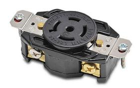
Bryant industrial heavy duty single locking blade receptacle, 20A, 277/480 VAC, 3-phase, 4-pole, 5-wire, NEMA L22-20, nylon molded housing, black.
