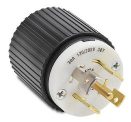
Bryant industrial heavy duty locking blade plug, 30A, 120/208 VAC, 3-phase, 4-pole, 5-wire, NEMA L21-30, accepts cord size 0.46-1.15in, nylon housing, black and white.
