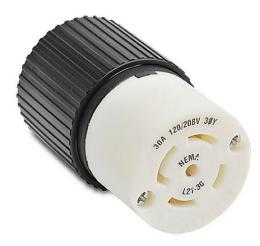
Bryant industrial heavy duty locking blade connector, 30A, 120/208 VAC, 3-phase, 4-pole, 5-wire, NEMA L21-30, accepts cord size 0.46-1.15in, nylon housing, black and white.
