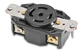
Bryant industrial heavy duty single locking blade receptacle, 30A, 120/208 VAC, 3-phase, 4-pole, 5-wire, NEMA L21-30, nylon molded housing, black.
