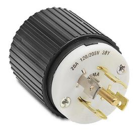
Bryant industrial heavy duty locking blade plug, 20A, 120/208 VAC, 3-phase, 4-pole, 5-wire, NEMA L21-20, accepts cord size 0.46-1.15in, nylon housing, black and white.
