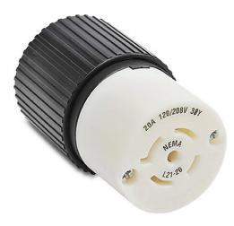
Bryant industrial heavy duty locking blade connector, 20A, 120/208 VAC, 3-phase, 4-pole, 5-wire, NEMA L21-20, accepts cord size 0.46-1.15in, nylon housing, black and white.
