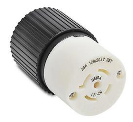
Bryant industrial heavy duty locking blade connector, 20A, 120/208 VAC, 3-phase, 4-pole, 5-wire, NEMA L21-20, accepts cord size 0.46-1.15in, nylon housing, black and white.
