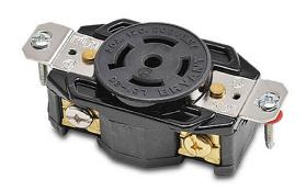
Bryant industrial heavy duty single locking blade receptacle, 20A, 120/208 VAC, 3-phase, 4-pole, 5-wire, NEMA L21-20, nylon molded housing, black.
