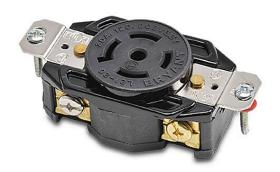
Bryant industrial heavy duty single locking blade receptacle, 20A, 120/208 VAC, 3-phase, 4-pole, 5-wire, NEMA L21-20, nylon molded housing, black.
