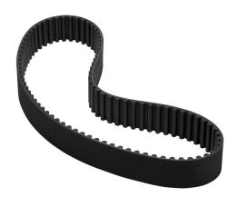
SureMotion timing belt, 8mm 8M pitch, 30mm wide, 90 tooth, 720mm pitch length (circumference), neoprene, fiberglass reinforced.
