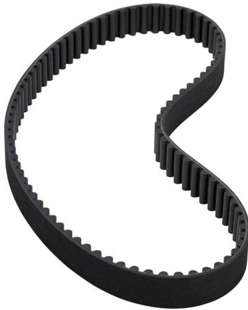
SureMotion timing belt, 8mm 8M pitch, 20mm wide, 90 tooth, 720mm pitch length (circumference), neoprene, fiberglass reinforced.
