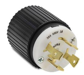
Bryant industrial heavy duty locking blade plug, 30A, 600 VAC, 3-phase, 3-pole, 4-wire, NEMA L17-30, accepts cord size 0.46-1.15in, nylon housing, black and white.
