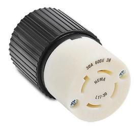
Bryant industrial heavy duty locking blade connector, 30A, 600 VAC, 3-phase, 3-pole, 4-wire, NEMA L17-30, accepts cord size 0.46-1.15in, nylon housing, black and white.
