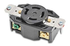
Bryant industrial heavy duty single locking blade receptacle, 30A, 600 VAC, 3-phase, 3-pole, 4-wire, NEMA L17-30, nylon molded housing, black.
