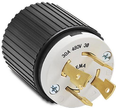
Bryant industrial heavy duty locking blade plug, 30A, 480 VAC, 3-phase, 3-pole, 4-wire, NEMA L16-30, accepts cord size 0.46-1.15in, nylon housing, black and white.
