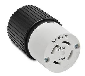
Bryant industrial heavy duty locking blade connector, 30A, 480 VAC, 3-phase, 3-pole, 4-wire, NEMA L16-30, accepts cord size 0.46-1.15in, nylon housing, black and white.
