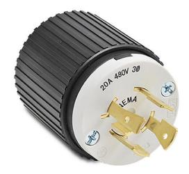
Bryant industrial heavy duty locking blade plug, 20A, 480 VAC, 3-phase, 3-pole, 4-wire, NEMA L16-20, accepts cord size 0.46-1.15in, nylon housing, black and white.
