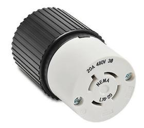
Bryant industrial heavy duty locking blade connector, 20A, 480 VAC, 3-phase, 3-pole, 4-wire, NEMA L16-20, accepts cord size 0.46-1.15in, nylon housing, black and white.
