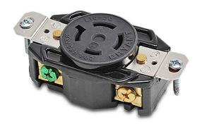
Bryant industrial heavy duty single locking blade receptacle, 20A, 480 VAC, 3-phase, 3-pole, 4-wire, NEMA L16-20, nylon molded housing, black.
