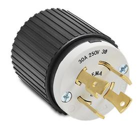
Bryant industrial heavy duty locking blade plug, 30A, 250 VAC, 3-phase, 3-pole, 4-wire, NEMA L15-30, accepts cord size 0.46-1.15in, nylon housing, black and white.
