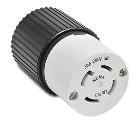
Bryant industrial heavy duty locking blade connector, 30A, 250 VAC, 3-phase, 3-pole, 4-wire, NEMA L15-30, accepts cord size 0.46-1.15in, nylon housing, black and white.
