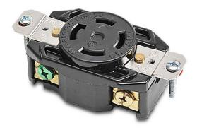
Bryant industrial heavy duty single locking blade receptacle, 30A, 250 VAC, 3-phase, 3-pole, 4-wire, NEMA L15-30, nylon molded housing, black.
