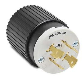
Bryant industrial heavy duty locking blade plug, 20A, 250 VAC, 3-phase, 3-pole, 4-wire, NEMA L15-20, accepts cord size 0.46-1.15in, nylon housing, black and white.
