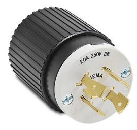
Bryant industrial heavy duty locking blade plug, 20A, 250 VAC, 3-phase, 3-pole, 4-wire, NEMA L15-20, accepts cord size 0.46-1.15in, nylon housing, black and white.
