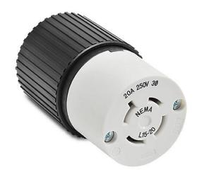
Bryant industrial heavy duty locking blade connector, 20A, 250 VAC, 3-phase, 3-pole, 4-wire, NEMA L15-20, accepts cord size 0.46-1.15in, nylon housing, black and white.
