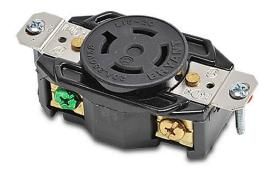
Bryant industrial heavy duty single locking blade receptacle, 20A, 250 VAC, 3-phase, 3-pole, 4-wire, NEMA L15-20, nylon molded housing, black.
