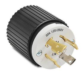
Bryant industrial heavy duty locking blade plug, 30A, 125/250 VAC, 1-phase, 3-pole, 4-wire, NEMA L14-30, accepts cord size 0.46-1.15in, nylon housing, black and white.
