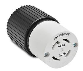
Bryant industrial heavy duty locking blade connector, 30A, 125/250 VAC, 1-phase, 3-pole, 4-wire, NEMA L14-30, accepts cord size 0.46-1.15in, nylon housing, black and white.
