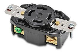
Bryant industrial heavy duty single locking blade receptacle, 30A, 125/250 VAC, 1-phase, 3-pole, 4-wire, NEMA L14-30, nylon molded housing, black.
