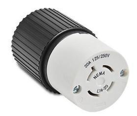
Bryant industrial heavy duty locking blade connector, 20A, 125/250 VAC, 1-phase, 3-pole, 4-wire, NEMA L14-20, accepts cord size 0.46-1.15in, nylon housing, black and white.
