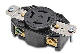
Bryant industrial heavy duty single locking blade receptacle, 20A, 125/250 VAC, 1-phase, 3-pole, 4-wire, NEMA L14-20, nylon molded housing, black.
