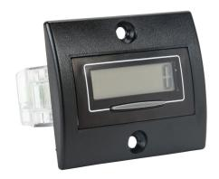
Trumeter electrical counter, 9mm 8-digit LCD, 5-110 VDC or 10-240 VAC input, remote, manual or disabled reset, rectangular flush mount with clip, screw terminals.
