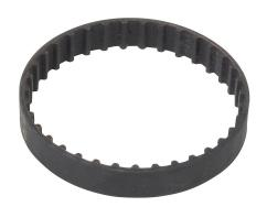
SureMotion timing belt, 1/5in XL pitch, 3/8in wide, 35 tooth, 7in pitch length (circumference), neoprene, fiberglass reinforced.
