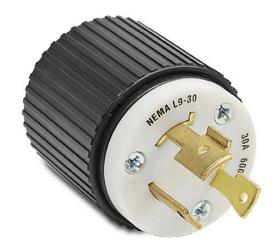
Bryant industrial heavy duty locking blade plug, 30A, 600 VAC, 1-phase, 2-pole, 3-wire, NEMA L9-30, accepts cord size 0.3-0.95in, nylon housing, black and white.
