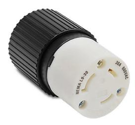
Bryant industrial heavy duty locking blade connector, 30A, 600 VAC, 1-phase, 2-pole, 3-wire, NEMA L9-30, accepts cord size 0.3-0.95in, nylon housing, black and white.
