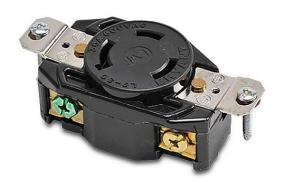
Bryant industrial heavy duty single locking blade receptacle, 30A, 600 VAC, 1-phase, 2-pole, 3-wire, NEMA L9-30, nylon molded housing, black.
