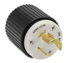
Bryant industrial heavy duty locking blade plug, 20A, 600 VAC, 1-phase, 2-pole, 3-wire, NEMA L9-20, accepts cord size 0.3-0.95in, nylon housing, black and white.
