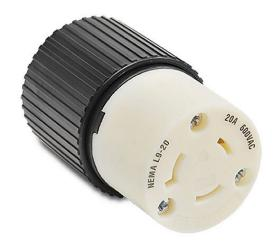
Bryant industrial heavy duty locking blade connector, 20A, 600 VAC, 1-phase, 2-pole, 3-wire, NEMA L9-20, accepts cord size 0.3-0.95in, nylon housing, black and white.
