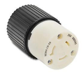
Bryant industrial heavy duty locking blade connector, 20A, 600 VAC, 1-phase, 2-pole, 3-wire, NEMA L9-20, accepts cord size 0.3-0.95in, nylon housing, black and white.
