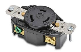
Bryant industrial heavy duty single locking blade receptacle, 20A, 600 VAC, 1-phase, 2-pole, 3-wire, NEMA L9-20, nylon molded housing, black.
