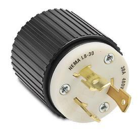
Bryant industrial heavy duty locking blade plug, 30A, 480 VAC, 1-phase, 2-pole, 3-wire, NEMA L8-30, accepts cord size 0.3-0.95in, nylon housing, black and white.
